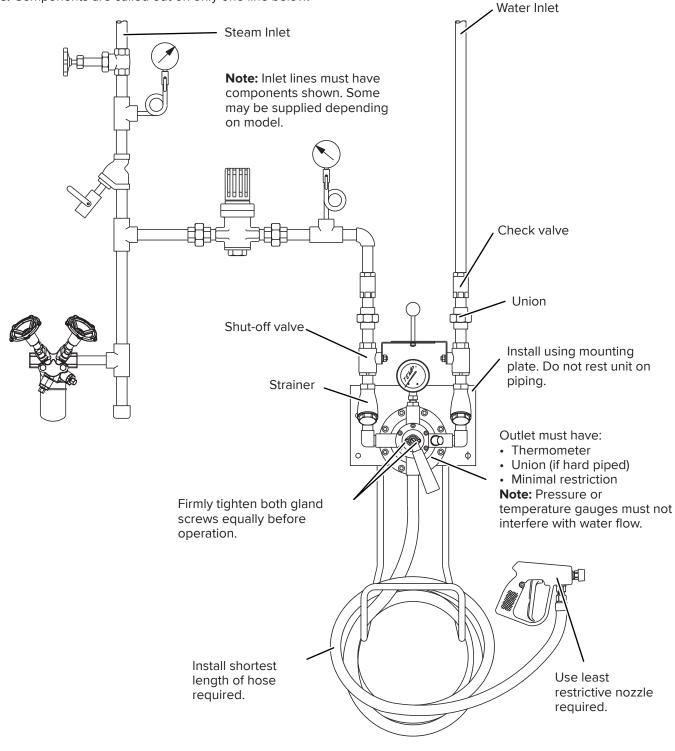
Note: Code or regulatory requirements may include back-flow preventers (single or double action) or vacuum breakers, which are not listed above.
