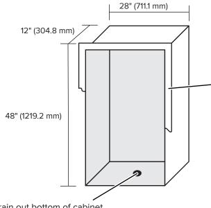
On flush mount cabinets mounting flange typically extends 2" (50.8 mm) beyond cabinet wall.
